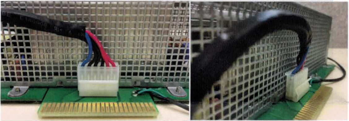
Figure 8: Detail of the PSU output cable connector, connected to the OCPA adapter
