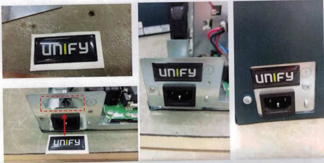
Figure 19: Placing the Unify logo label (V32905-A3-X652) at the open hole of the system housing
