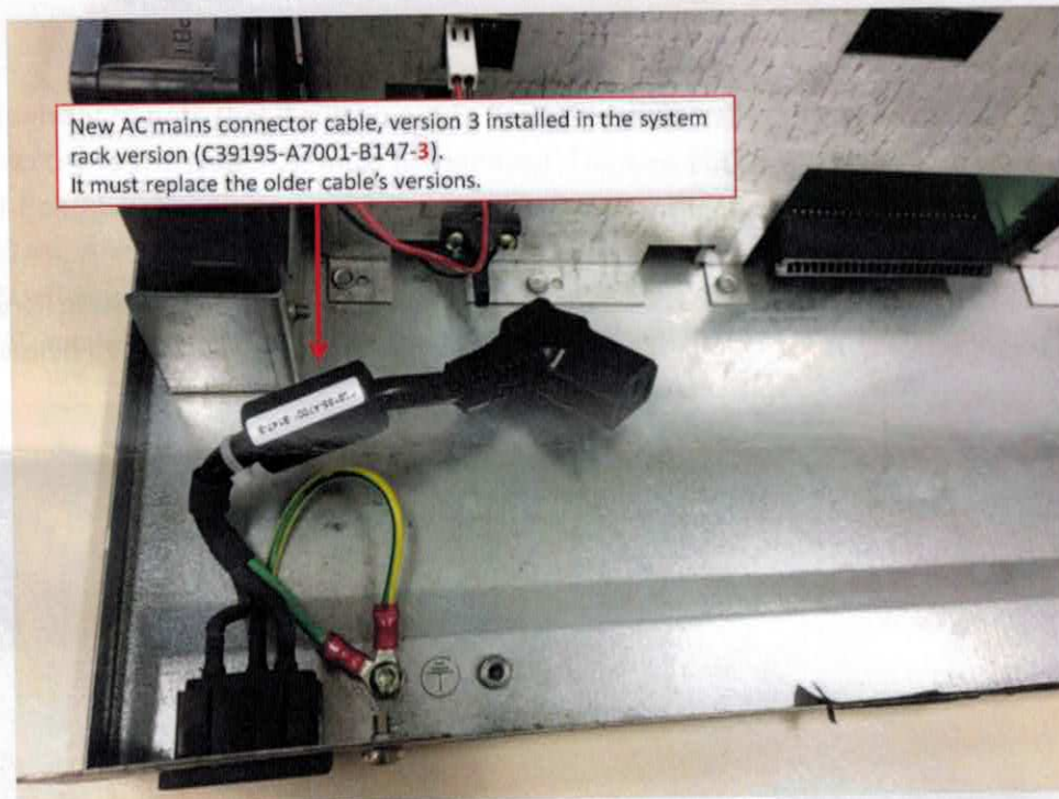
Figure 8: Replacing the mains AC connector cable (C39195-A7001-B147) to the latest version
