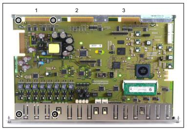
OpenScape Business X3W and X5W STRB is inserted in option 1 of slot level 3 (X3W) or 6 (X5W) with the component side facing upwards. The electrical connection to the OCCM mainboard (OBUS plug contact) is established via the optional adapter cable OPAL (C39195-A7001-B130).
