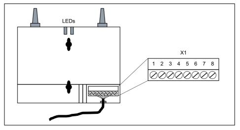
Figure: Rear View - Terminal Strip X1
