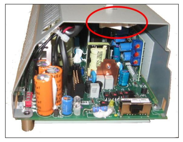
8) Connect the fan power cable to the open side of the UPSC-D power supply.
