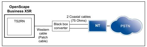
The following cable types can be used to connect to the network terminator NT:
