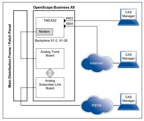
Figure: TMCAS2 – Ways to Access the Board
