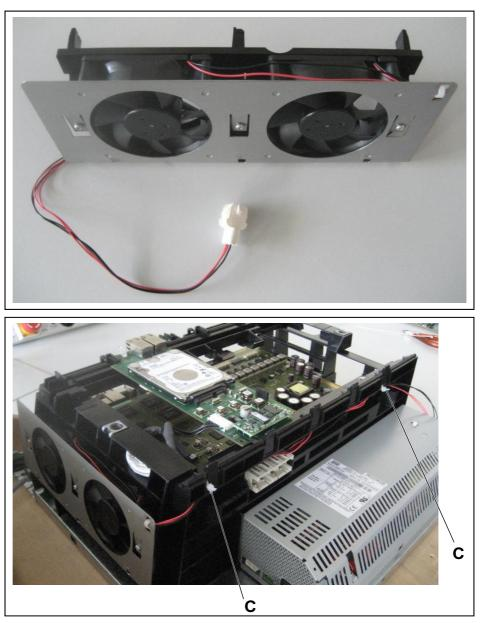
7) Fix the fan power cable to the housing with the two cable ties (C) supplied.
