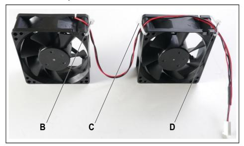
*g)* Insert the two new fans into the brackets provided for this purpose and fix the fans to the brackets with the supplied screws (E, F, G and H). Pay special attention to the correct air flow direction, which is indicated by arrows on the fan housing (the arrows point into the system, i.e., the cold air must be blown into the system).
