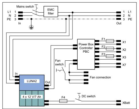
**Figure:** OpenScape Business Powerbox – Block diagram with four 12V 7Ah batteries and LUNA2 power supply
