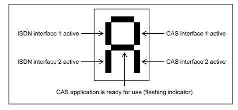
Figure: TMCAS2 - Statuses of the Interfaces and the CAS Application
