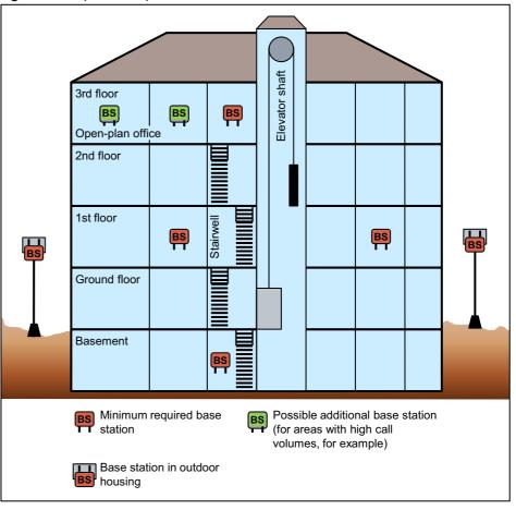
Figure: Example for the placement of base stations outdoors
