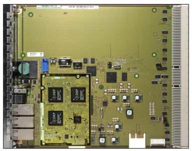
Figure: OCCB subboard mounted on OCCL
