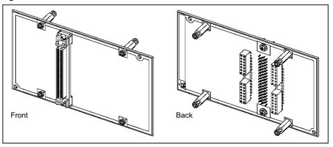
Figure: DBSAP - Installation on the Backplane of the Expansion Box
