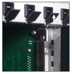
2) Slide the gray board latch into the board frame and press it firmly into the anchor.
