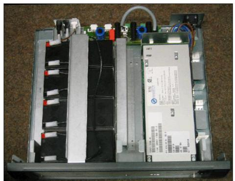
**NOTICE:** When storing an OpenScape Business Powerbox equipped with batteries or during prolonged periods of non-operation, the F4 fuse (protection for XBatt output) must be removed.
