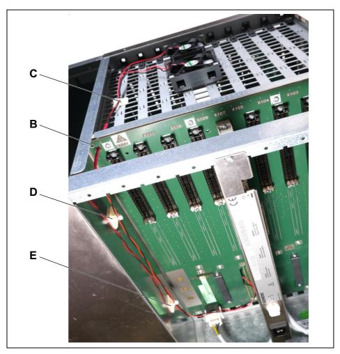
*j)* Connect the two power cable plugs to the X117 backplane connector. Note that the red plug must be connected to the first left pin from the top, and the black plug to the fifth left pin from the top. Make sure that sufficient distance from the internal 230V wiring is maintained.
