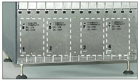
From a technical viewpoint, there are no differences between the slots. The LUNA2 modules can be used in all slots, regardless of the selected operating mode. However, to ensure optimal ventilation, there should be at least one free slot between two LUNA2 modules if possible. To achieve a uniform LUNA2 configuration of the communication systems worldwide, the following rules should be observed:
