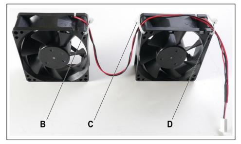
9) Insert the two new fans into the brackets provided for this purpose and fix the fans to the brackets with the supplied screws (E, F, G and H). Pay special attention to the correct air flow direction, which is indicated by arrows on the fan housing (the arrows point into the system, i.e., the cold air must be blown into the system).
