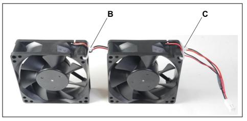
*g)* Insert the two new fans into the brackets provided for this purpose. Pay special attention to the correct air flow direction, which is indicated by arrows on the fan housing (the arrows point into the system, i.e., the cold air must be blown into the system).
