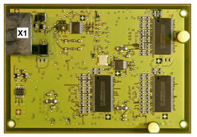
7) Insert the PCI-E connector X1 of the OCCB subboard (component side down) onto the X6 edge connector of the OCCL mainboard. Make sure that the two spacing bolts are plugged into the appropriate holes on the mainboard.
