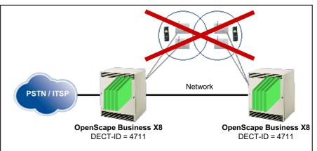
Identical DECT IDs and overlapping radio areas result in incorrect handover causing a breakdown in communication.
