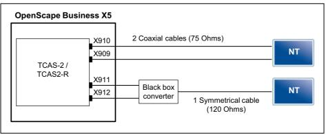
The following cable types can be used to connect to the network terminator NT:
