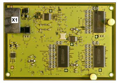
6) Insert the PCI-E connector X1 of the desired OCCB subboard (component side down) onto the X18 edge connector of the OCCMR mainboard. Make
