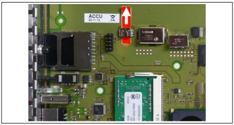
Figure: OCCL - Battery with protective film
