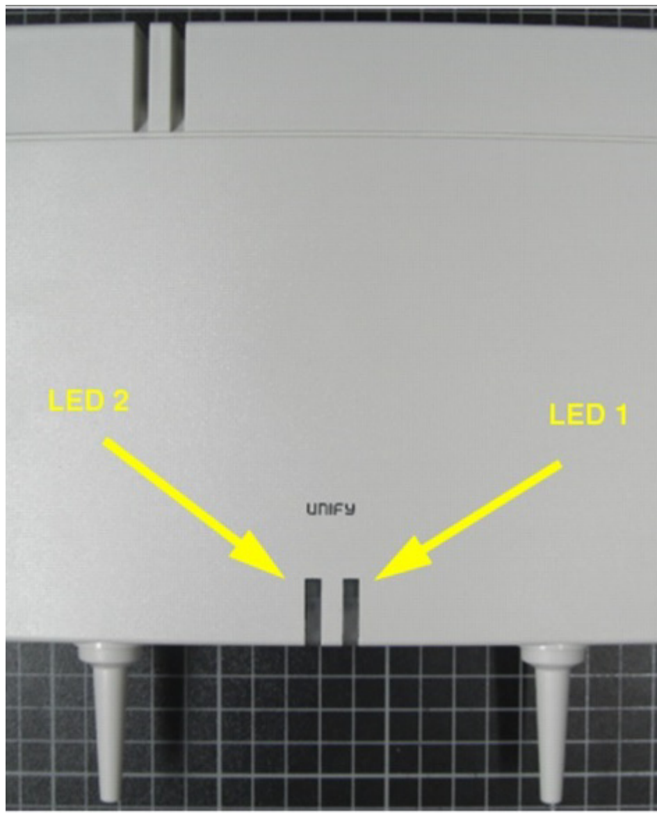
Figure: Base Station BS5
