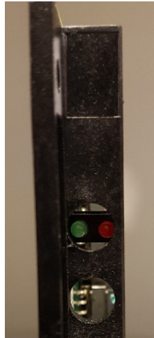
Figure: SLMU – LEDs on the Front Panel
