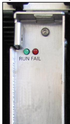
Figure: SLCN – LEDs on the Front Panel
