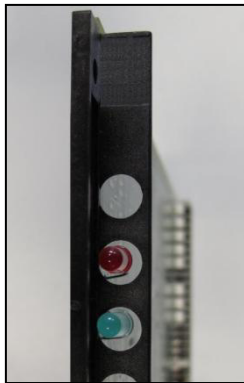
Figure: TMDID – LEDs on the Front Panel
