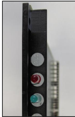
Figure: SLMO8N, SLMO24N – LEDs on the Front Panel
