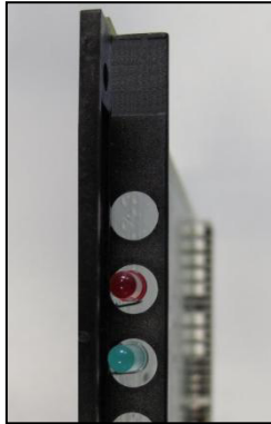
Figure: SLMAV8N, SLMAV24N – LEDs on the Front Panel
