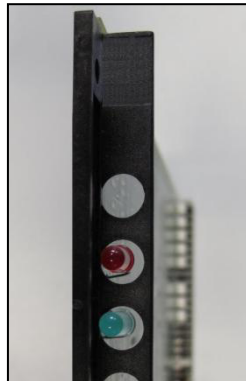
Figure: STMD3 – LEDs on the Front Panel
