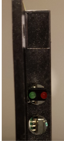
Figure: SLMU – LEDs on the Front Panel
