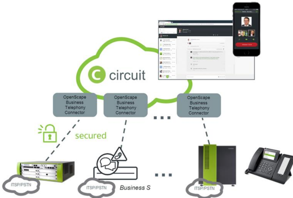
Figure 40 OpenScape Business Connection to Circuit
