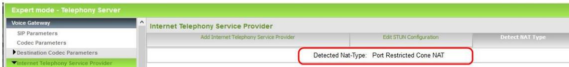
Note: The NAT type detection of the OpenScape Business (may falsely detect the NAT type of the Company router as "Symmetric NAT" if outbound IP traffic is restricted in the Company router. Please make sure that the ports listed above are open in outbound direction as well.
